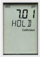
• Freeze readings Press the SET/HOLD button to hold readings on the display
