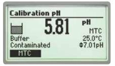
Buffer Contaminated –The offset of the electrode is not in the accepted range. Check if the electrode is broken or clean it following the Cleaning Procedure at the end of this section. Check the quality of the buffer. If necessary, change the buffer.
