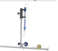
It consists of a rail on which a low-friction cylinder can slide. By rotating the device, it is possible to read on the spring scale, the value of the centrifugal force, and it is possible to check the centrifugal force formula.
