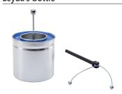
Cylindrical condenser for experiments on the electric capacity. It is supplied with insulated handle to extract the inner framework when the condenser is charged.
