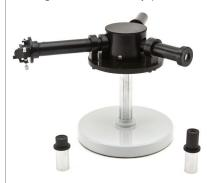
prism made of highly dispersive material. With this device you can study the spectrum of a source of monochromatic or polychromatic light. We recommend the use of interferential filters to the check of the wavelength.
