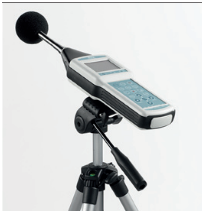
Noise Studio: NS5 "Environmental Noise" module; sound sources analysis with tonality and impulsiveness evaluation.
