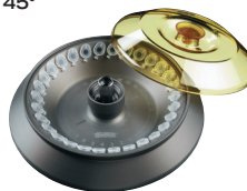
Angle rotor, 30-place, Cat. No. 02430B n = 15,000 \text{ min}^{-1} max RCF 20.376 Lid OE3243 incl.
