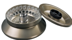
Angle rotor, 24-place Cat. No. 02428 n = 15,000 \text{ min}^{-1} , max RCF 21,382 Lid with bio-containment, autoclavable, phenol-re- sistant incl.
