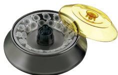
Angle rotor, 30-place, Cat. No. 02427A n = 15,000 \text{ min}^{-1} , max RCF 20.627 Lid OE3243 incl.
