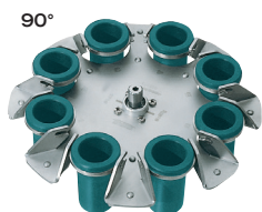
Swing-out rotor, 8-place, for 8 x 15 ml, n= 4,000 min -1 , RCF 2,415 Stainless steel, with suspensions No. 01644, PA, fibreglass reinforced.
