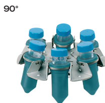
Swing-out rotor, 6-place, for 6 x 50/15 ml Falcon tubes n= 4,000 min -1 , RCF 2,701, Stainless steel, with suspensions, PA, fiber- glass reinforced.
