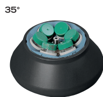
Angle rotor, 6-place, Cat. No. 01620A n= 6,000 min -1 , max. RCF 4,226 illustrated with adapter set 01646
