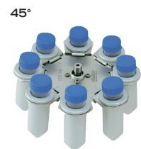
Swing-out rotor, 8-place, for 8 x 50/15 ml Falcon tubes n= 4,000 min -1 , RCF 2,469 stainless steel, with suspensions, aluminium.
