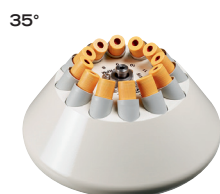
Angle rotor, 12-place, Cat. No. 01613 n= 6,000 min -1 , max. RCF 4,146
